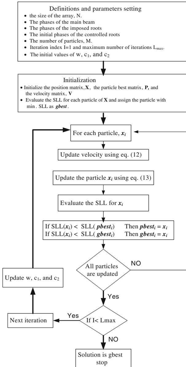
**Fig. 3** Flow chart of the PSO algorithm
