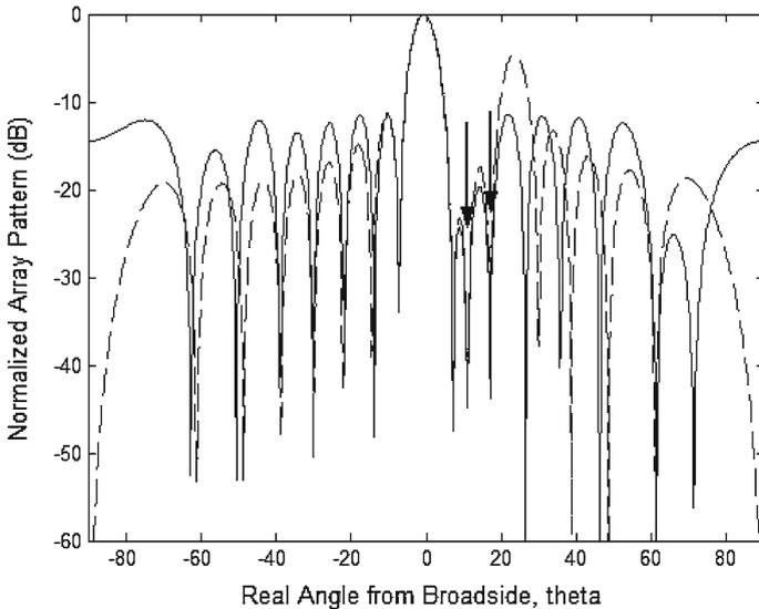
**Fig. 4** The optimized array pattern with two nulls imposed at  $\theta_1 = 11^\circ$  and  $\theta_2 = 17^\circ$  (Solid). The array pattern when the two nulls are imposed at the array pattern of a uniformly excited linear array,  $N = 16$ ,  $d_0 = \lambda/2$  (Dotted)
