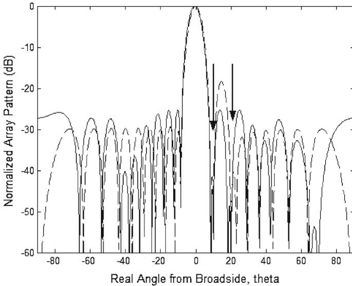
**Fig. 6** The optimized array pattern with two nulls imposed at  $\theta_1 = 10^\circ$  and  $\theta_2 = 20^\circ$ . and  $(\psi_{n,1} = 31.26^\circ$  and  $\psi_{n,2} = 61.56^\circ)$  (Solid). The array pattern when the two nulls are imposed at the array pattern of a 30 dB Chebyshev array,  $N = 20$ ,  $d_0 = \lambda/2$  (Dotted)
