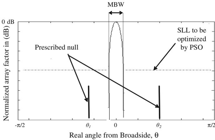
**Fig. 2** The objective function with two nulls imposed at a given arbitrary directions using the array polynomial and optimal SLL by PSO
